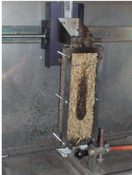
Procedure according to EN ISO 11925-2 / The Single Flame Source Test
